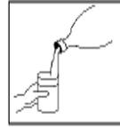
Unscrew the flask and fill it with water up to the line (see humidifier instructions). Then screw the lid on the humidifier flask until there are no leaks.
